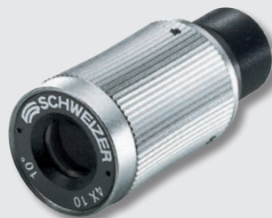
931945 Kepler 4x10 Magnification 4x, field of view 10,0°, objective Ø 10 mm
