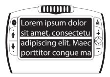
2. Press and HOLD the green/yellow button • and then press the yellow PLUS button • or the yellow MINUS button • to move the reading line up or down.
